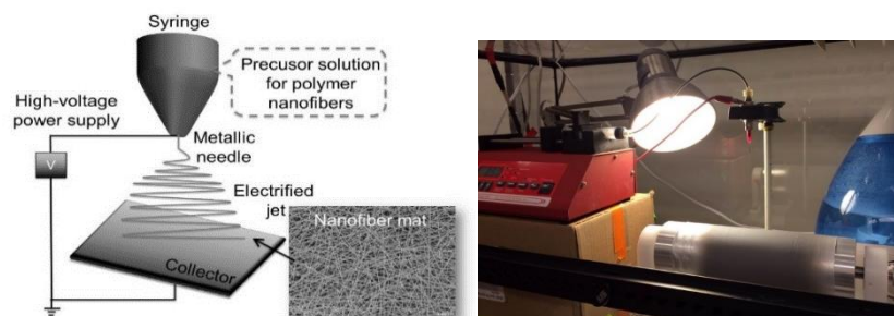
Figure 1-9. Set-up of the lab electrospinning apparatus
